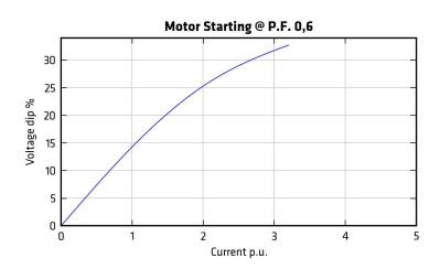
Motor starting curve locked rotor (0,3PF)
