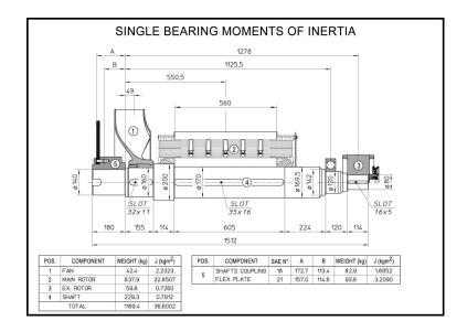
Alternator ref. KH04590T Alternator type KH04590TO4D
