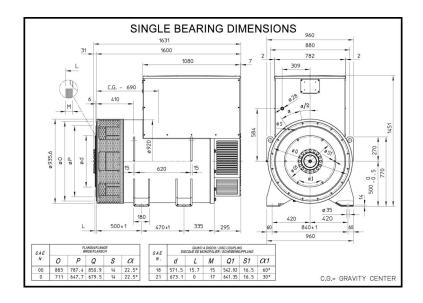
Alternator ref. KH04590T Alternator type KH04590TO4D
