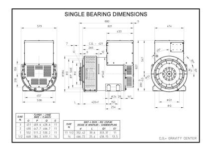
Alternator ref. Alternator type KH01180T KH01180TO4D
