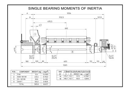
Alternator ref. KH03544T Alternator type KH03544TO4D
