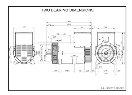
Alternator ref. KH03544T Alternator type KH03544TO4D
