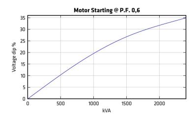
Motor starting curve locked rotor (0,3PF)
