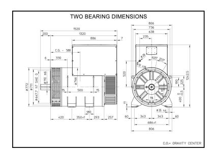
Alternator ref. KH02970T Alternator type KH02970TO4D
