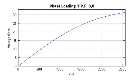
Alternator ref. KH02970T Alternator type KH02970TO4D
