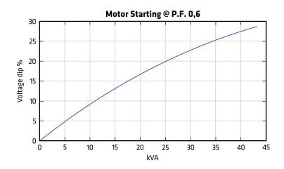
Motor starting curve locked rotor (0,3PF)
