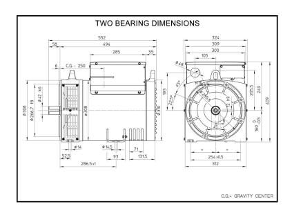
Alternator ref. KH00404T Alternator type KH00404TO4N
