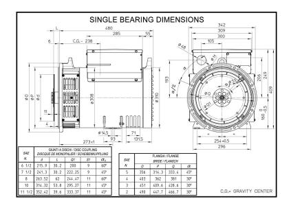
Alternator ref. KH00404T Alternator type KH00404TO4N
